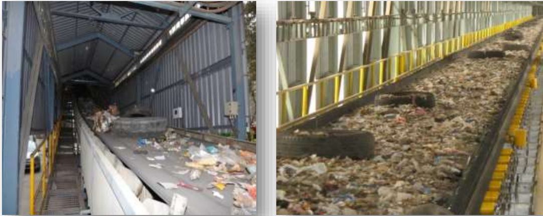
Fig: RDF & waste tyre handling system
